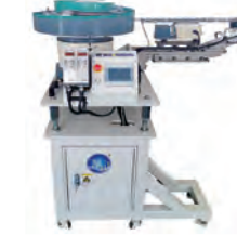
Housing inserting station
